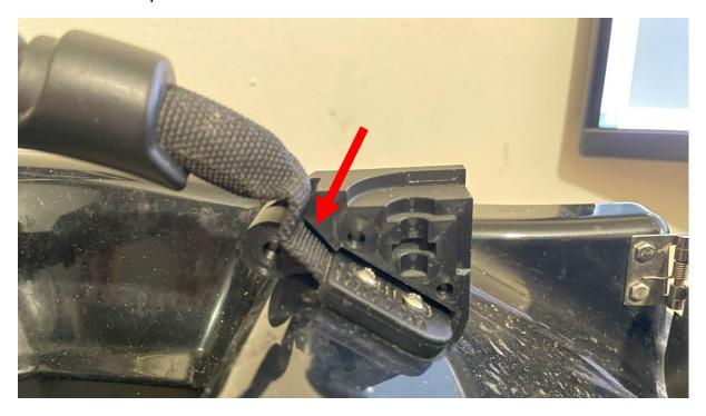
You can see the handle passes through a cut-out in the bracket, indicated by red arrow.
