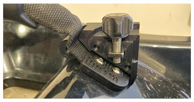
Next Step is to take the other side of the clamping bracket and slide it over the handle, squeezing the two parts together:
