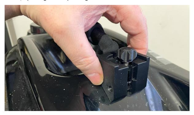
Squeeze it until the mounting bracket is nearly joined, you can then unscrew the M6 thumbscrew and the nut will be held in place.
