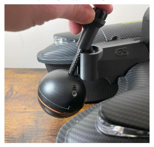
Then drop the tube and insert into the mount, the insert sits flush with the top of the mount when its fitted correctly.
