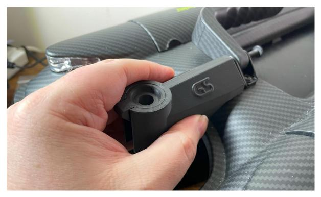
Next slowly screw the new handle screw into the mount, the mount should be drawn towards the handle bracket once the screw is sufficiently into the mount:
