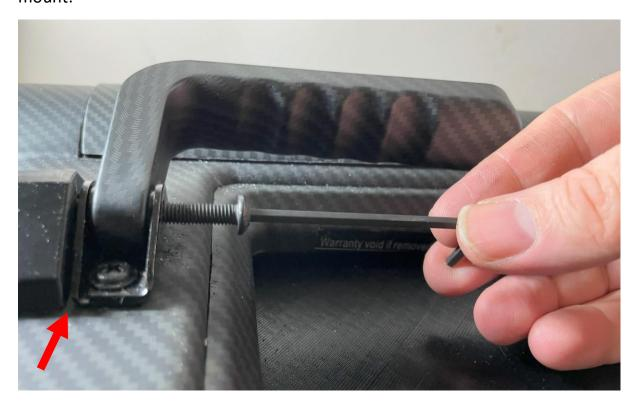
PLEASE NOTE — Do not over tighten the mounting screw - only use the small angle of the allen key for tightening the mount up, there is no need for excessive pressure here, the plastic will keep the screw in place nicely without it coming out.
