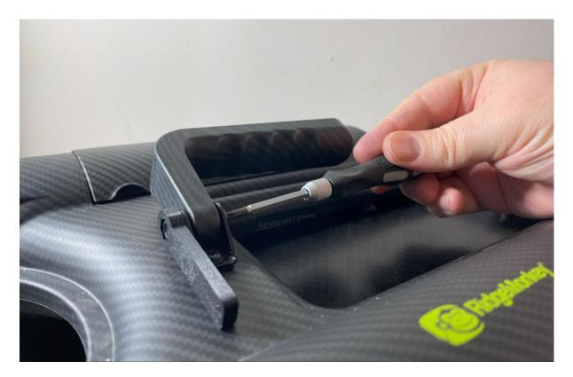
Next unscrew the M5x35 Button Head allen screw from the main housing (should be finger tight), once removed screw it into the hole until the thread is just protruding through the handle mounting plate by a few millimeters :
