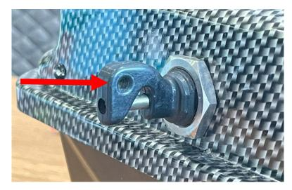
Please check there is no obstructions in the hole, if there is please screw the M4x22mm Screw into the hole – this should push out any moldings / rubbish from the hole.
