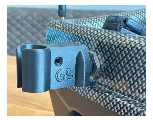
Slide it on until its fully seated against the hull of the boat, visually check the countersunk hole is aligned with the hole in the hook release. Due to some molding variations of the hook release the body was designed to be tight up against the body – therefore there maybe up to ½ hole misalignment.
