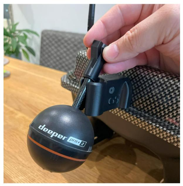
Then lower the sliding piece down whilst aligning the tab into the cut-out, press the sliding piece down (very slight click is felt).
